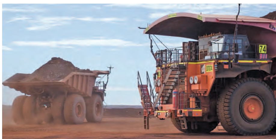
Autonomous Cat 793 and Hitachi EH5000 trucks at Roy Hill mine running on ASI Mining system
